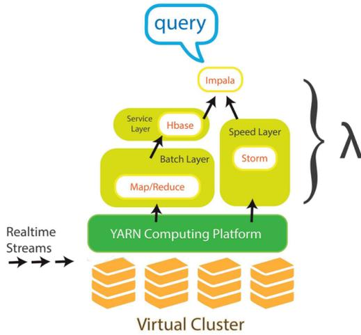
Fig. 3. REALICS Lambda based configuration. Tools from the Cloudera Hadoop ecosystem are placed in the corresponding layers of Lambda. The tools outlined in this figure are only indicative
